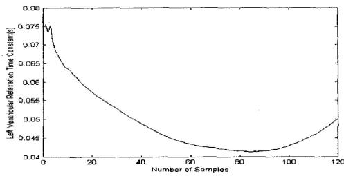
Fig. 1. Typical change of  $\tau$  as the ending point of IRP moves from the negative peak point of  $dP(t)/dt$  by one data point.  $\tau$  varies widely according to the location of the ending point of IRP.
