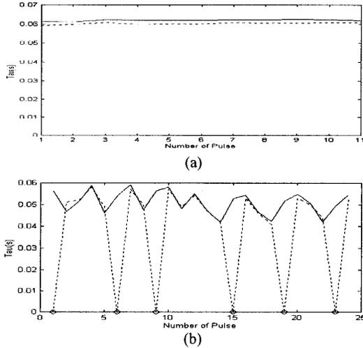
Fig. 4. Comparison between  $\tau$  obtained from Paulus et al's method and from proposed method. Solid line is for proposed method and dotted line is for Paulus et al's method. (a) uniform  $\tau$ , (b) variable  $\tau$ . Small circles indicate missed beats.
