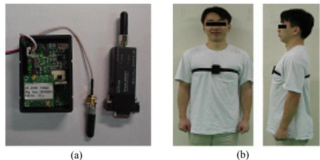
Fig. 1. Our ambulatory system for fall detection. (a) The developed system and Bluetooth module, (b) The system attached on chest with a belt.
