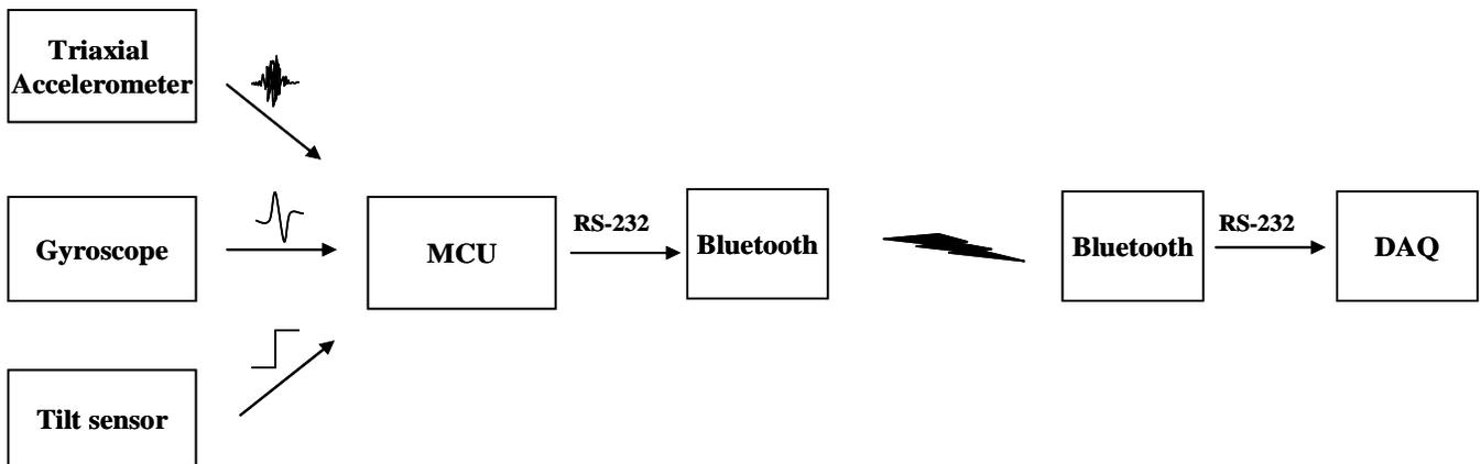
Fig. 2. Real-time monitoring system for fall detection. Triaxial accelerometer measures kinetic force, gyroscope estimates posture transition, and tilt sensor switches on when people is supine. Each data obtained from the sensors is converted to digital signal by microcontroller (AVR4433), and then the signal is transmitted to DAQ through Bluetooth Module.
