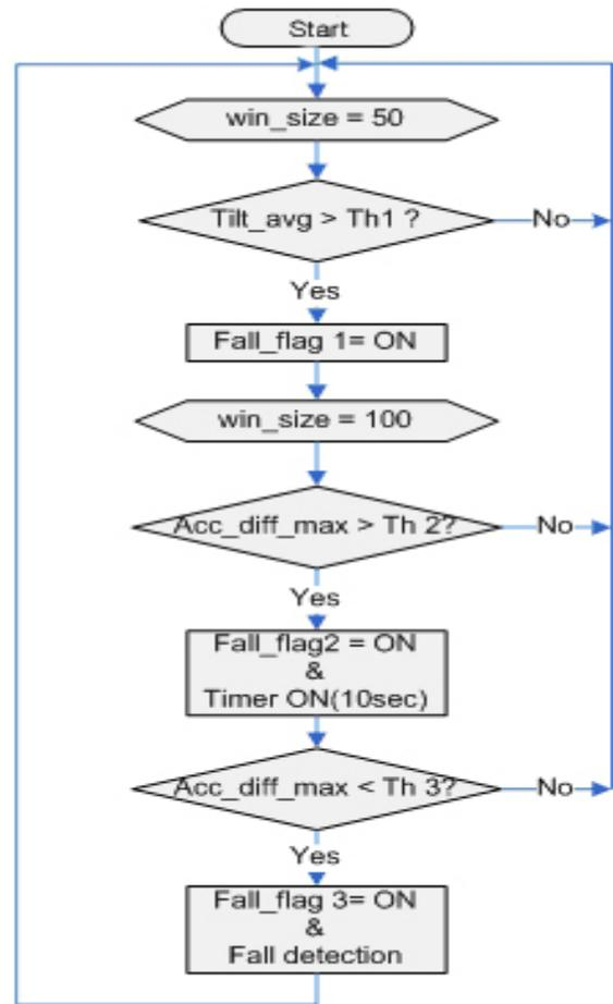
Fig. 3. Algorithm flow chart. If average value of buffered tilt signal in the window1 of size 50 is over threshold 1( $\alpha$ ), Fall\_flag1 becomes ON. After acceleration signals of each axe direction is differenced, if Maximum value among the buffered acceleration values in the window2 of size 100 is over Threshold 2( $\beta$ ), Fall\_flag2 become ON. When Timer is expired, if the Maximum value in window2 is below Threshold 3( $\gamma$ ), Falling become detected.
