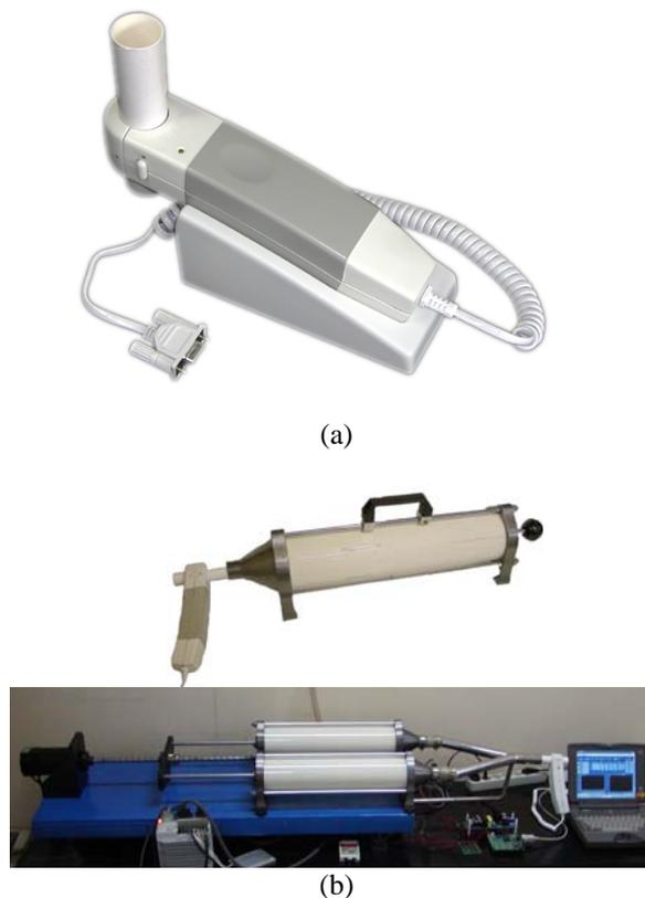
Figure 3: Pictures of (a) the developed spirometer and (b) the 3L syringe with a motor driven flow generator.
