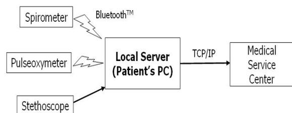
Figure 2: Functional block diagram of the developed system.
