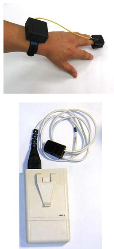
Figure 4: Developed two pulse oxymeters of the wrist-worn type and the waist-worn type.
