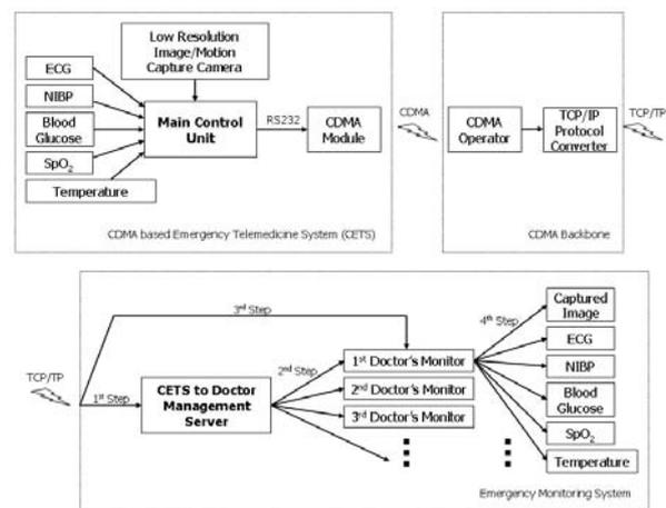
Figure 3: Functional block diagram of the total emergency healthcare service system including the CETS
