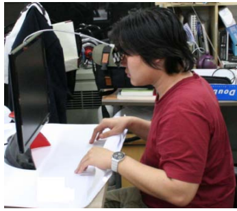
Fig. 13. The 3D viewer unit consisted of LCD monitor and stereoscope.
