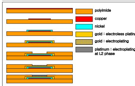
Figure 4. Image of film type electrode.
