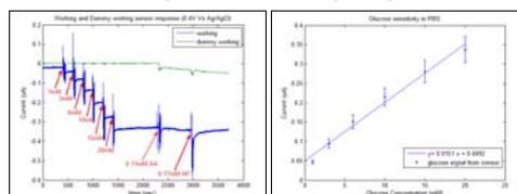
Figure 5. Working electrode responded to glucose selectively. 5 independent sensor response was collected and plotted. The R<sup>2</sup> was 0.98.
