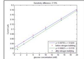
Figure 6. Sensor was not affected by the O<sub>2</sub> concentration. Difference between sensitivity in N<sub>2</sub> saturated solution and O<sub>2</sub> resolved solution was less than 4 percent.
