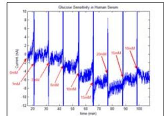
Figure 8. Sensor sensitivity for glucose in human serum. Whole blood was sampled and leaved in autoclave to drop the glucose concentration to zero then centrifuged.
