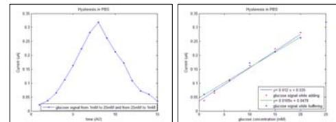
Figure 7. Hysteresis characteristic of the sensor was applicable. Difference between sensitivity in glucose adding and PBS dilution signal was less than 10 percent.
