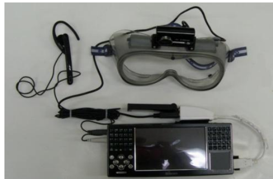
Fig. 1. Developed EVAT system consisting of a PC cam on a protection goggle, a UMPC, and a mic-earphone set
