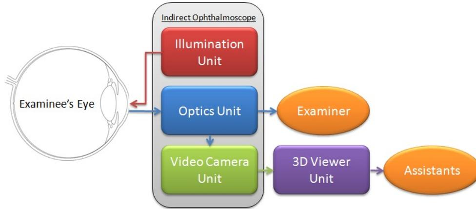
Fig. 3. Block diagram of our BIO system which consists of illumination, optics, video camera and 3D viewer units.
