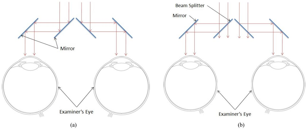
Fig. 6. Optics unit: schematic representations of the conventional BIO (a) and ours (b).
