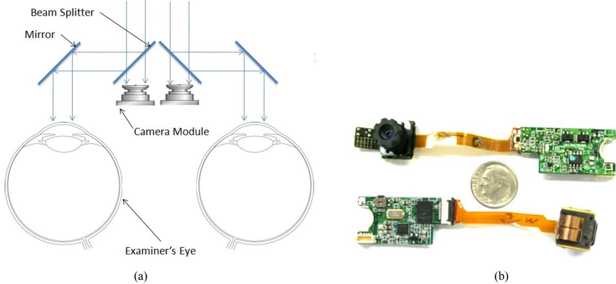
Fig. 8. Video camera unit: schematic representations of our BIO (a) and real picture of used camera modules (b).
