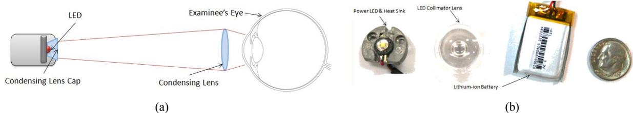
Fig. 4. Illumination unit: illumination process (a) and real picture of used components (b)
