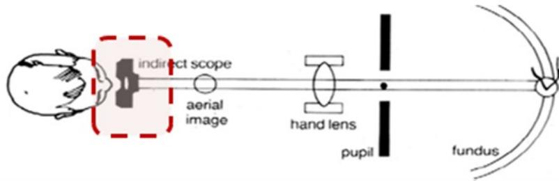
Fig.5. Optics unit composed of binocular eyepieces and hand-held condensing lens
