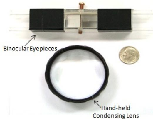
Fig.7. Optics unit: real pictures of binocular eyepiece (upper) and 20 diopter condensing lens (lower)
