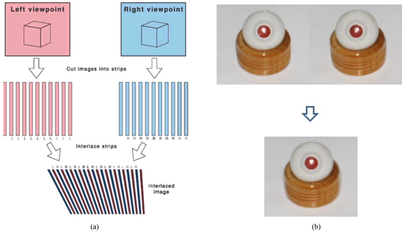
Fig. 9. Procedure making interlaced image from side-by-side image (stereo-pair image) (a) and example of autostereoscopic image for 3D LCD (b)
