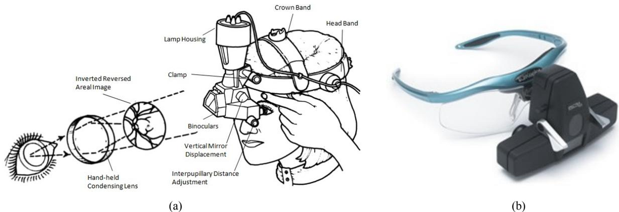
Fig. 2. Conventional binocular indirect ophthalmoscope (BIO) (a) and portable glasses-type BIO released recently (b)
