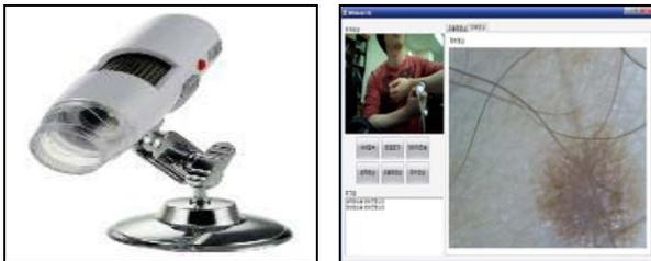
Fig. 8. USB digital microscope devices and application program
