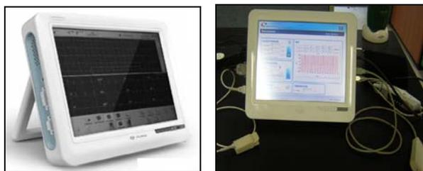
Fig. 5. ECG device (HiCare Dr. U) and application program
