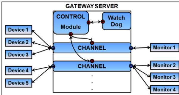
Fig. 1. Organization and data flow of the system. Device can be various health monitoring devices and monitor means medical caregiver.
