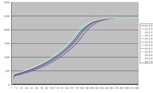
Fig 2 characteristic I-V Sigmoid curve of LAPS
