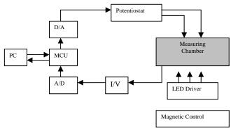
Fig 3 Block Diagram
