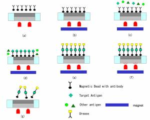
Fig 4. Magnetic bead based Separation
