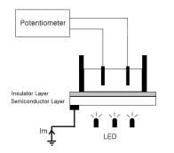
Fig 1 schematic diagram of LAPS system
