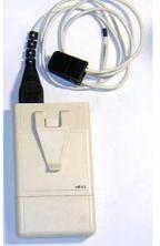
Figure 4: Developed two pulse oxymeters of the wristworn type and the waist-worn type. Performance of the developed  $SpO_2$  module was verified using a commercial  $SpO_2$  simulator (Oxitest plus7, DNI Nevada Inc, USA).
