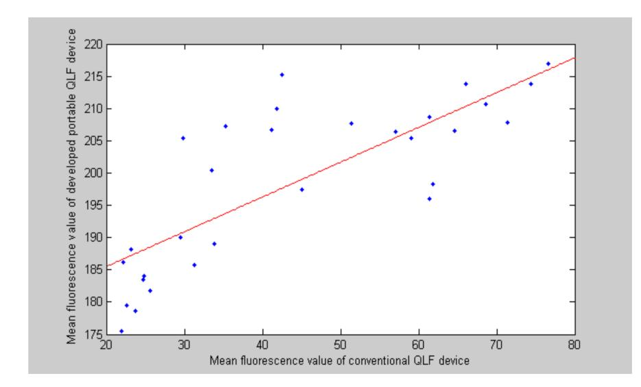
• The measured green fluorescence intensity values from two devices were strongly correlated (r = 0.79)
