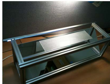
Figure 4. Picture of modified CatWalk setup. Polymer sheet in this picture is PDMS sheet instead of electrospun nanofiber sheet used for experiments.
